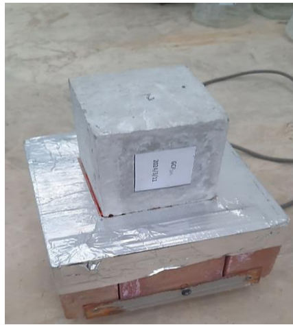
Fig. 7. Mechanism for measuring thermal conductivity of concrete samples
