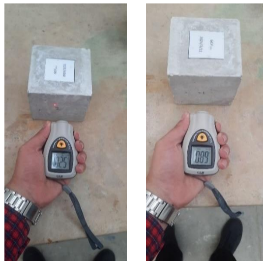
Fig. 8. Measurement of the temperature difference for the first group of mixtures (GCP 50% )
