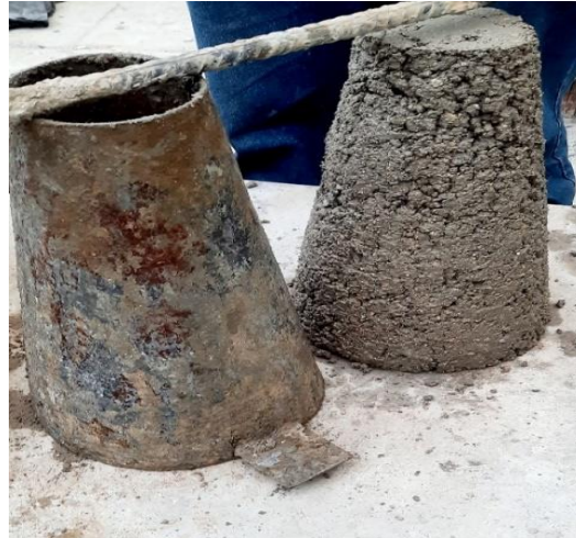
Fig. 5. Measurement of subsidence by the Abrams cone method for concrete mixture
